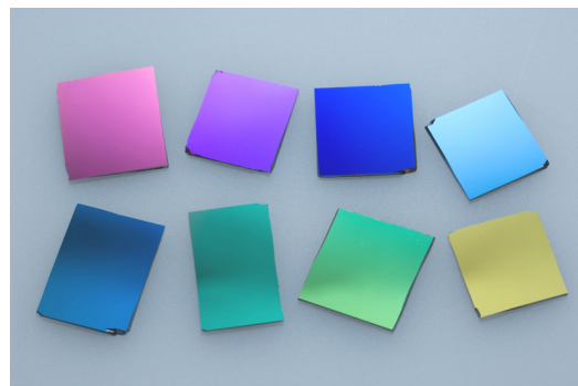
Figure 5.32: Al-Si-N coatings on pieces of silicon wafers. The colors are related to the thickness of the coatings, except for the yellow, that is a result of nitrogen deficiency during deposition. It was found that violet corresponds to 50 \text{ nm} film thickness, blue to \sim 200 \text{ nm} , green to \sim 500 \text{ nm} and pink to \sim 800 \text{ nm} , seemingly independent on the exact Al-Si-N film composition.
