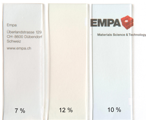
Figure 5.31: Al-Si-N coatings on glass show a good transparency, as seen from the printed text in the background. The slight shades of color are caused by interference effects which are related to small variations in the thickness of the coatings (about 1 \mu\text{m} ). The silicon content in at.% is indicated on the picture. It has however no influence on the colors seen here.
