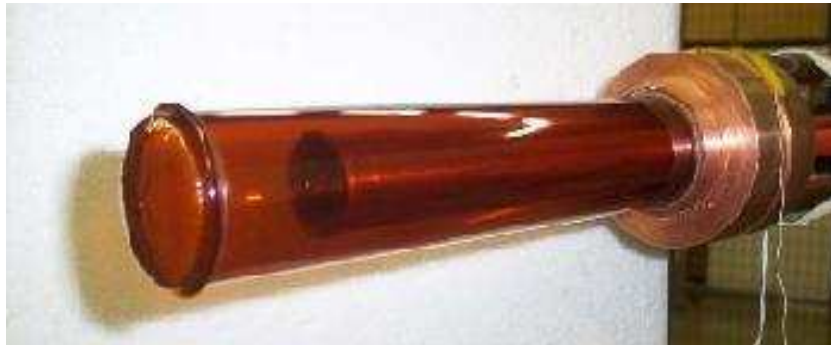
Figure 3.9: The Liquid Hydrogen Target
