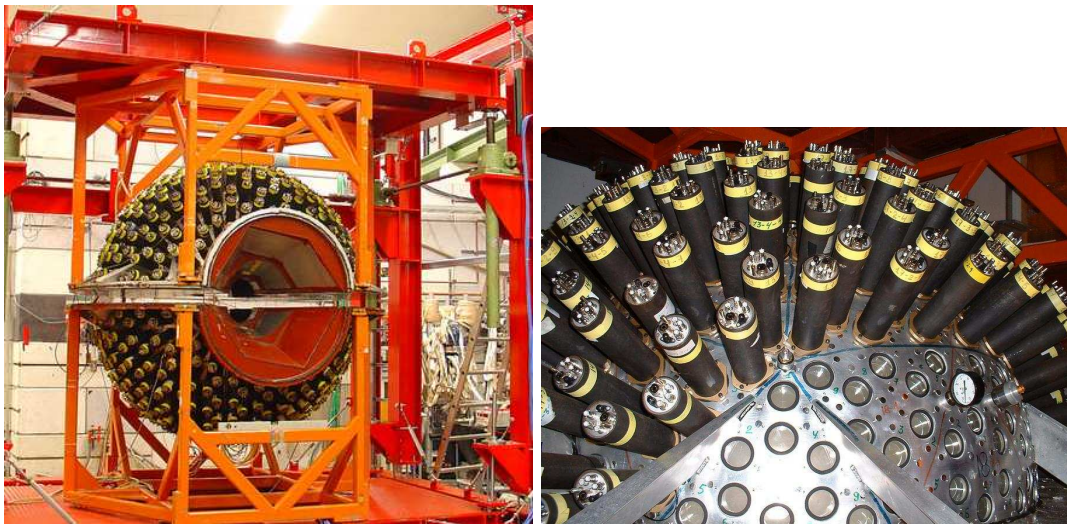
Figure 3.11: LEFT: Complete crystal ball before cabling. RIGHT: Part of the crystal ball detector. View of bare crystals and ones equipped with photomultipliers
