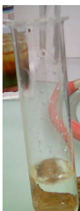
Figure 5.1 Droplets on the glass wall indicating a low wetting effect of 24 in dichloromethane in a test tube.
