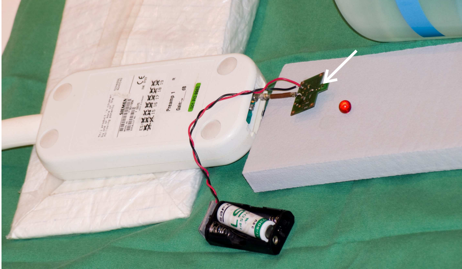
Figure 5.3: Photograph of the connection of the microcoil including connection to clinical scanner through flex coil small interface. The white arrow indicates the position of the micro-coil. The glycerol nitrate capsule (red ball) can be clearly seen.
