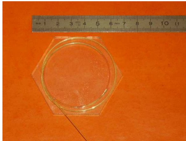
Figure 3.9: A picture of the veto detector. The hexagonal 5 mm plastic scintillator and its fiber guide.
