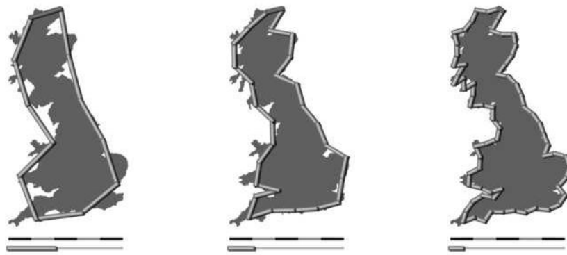
Figure 3.42: Example of fractal problem in nature: how long is the coast of Britain? Three different measurement of the same map with three different ruler sizes are shown. [29]
