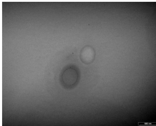
Figure 3.10. TEM micrograph of unstained A_5G_7 - b - PB_{5000} in PBS buffer, showing only single vesicles.
