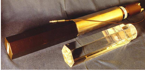
Figure 3.13: Each TAPS element is made of a 25 cm BaF2 crystal corresponding to 12 radiation lengths. The main part of the crystal is hexagonal, with a 2.5 cm end cylinder connected directly to a photomultiplier for read-out.
