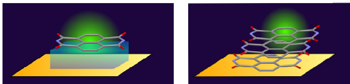
Figure 23: Strategies for decoupling the chromophore from the surface, either by an insulating salt layer (left) or by multilayers (right).
