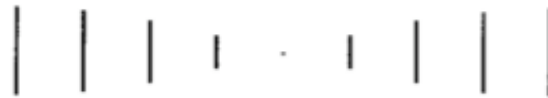
Figure 4.3: Electric-field picture for a single fringe of an IG (in which the excitation beams have parallel polarizations). The polarization of the electric field is constant across the grating, but the field amplitude is sinusoidally modulated.
