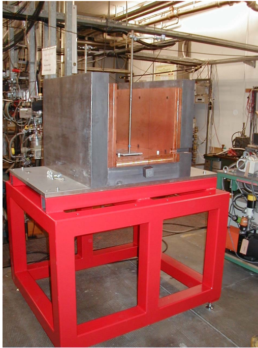
Figure 2.33: Shielding housing on the stand without detector, roof and doors. View from the back.
