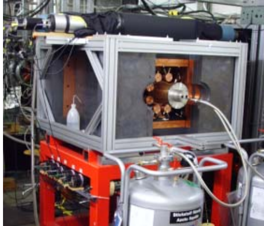
Figure 2.31: Bars of the cosmic rays detector placed on top of the shielding housing. The bars were additionally covered with black paper and draperies to prevent any infiltration of light into the scintillators, since the original cover was holey.
