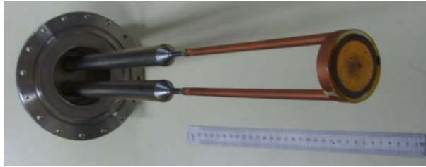
Figure 2.18: The beryllium foil with circular gold coating is cooled via liquid N 2 . The pipes for the nitrogen are connected to two cryogenic reservoirs. The picture was taken at the end of the experiment. The coating shows a degradation, which is due to the fact that a gold coating does not stick well on beryllium. In addition the thermal stress during the production and unfreezing of the ice targets of the measurement enhances the degradation.
