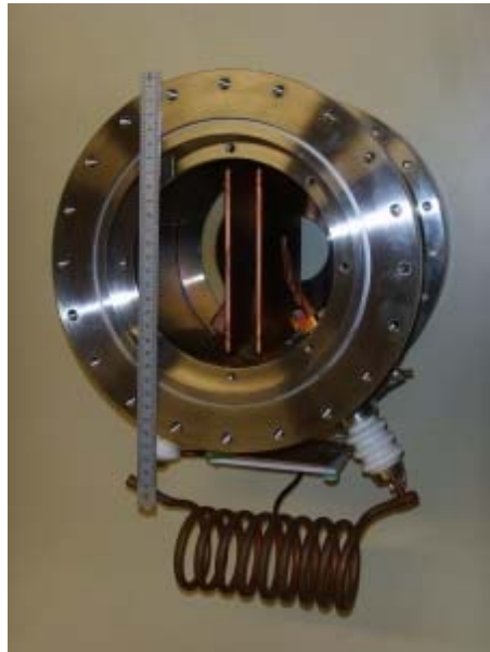
Figure 2.7: Steel barrel containing the copper plates of the beam chopper. The plates are 125 mm wide (in direction of the beam), 135 mm in height and 5 mm thick. The parallel plates are electrically isolated and at distance of 2 cm.
