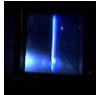
Figure 2.8: The beam is hitting a quartz and through scintillation and luminescence revealing its position.
