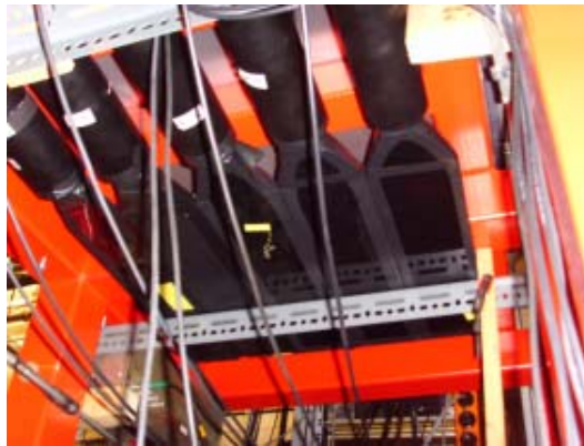
Figure 2.30: Paddles of the cosmic rays detector under the shielding housing. The beam is coming from left.
