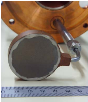
Figure 2.16: The \text{D}_2 -gas sprinkler consists of a porous metal sheet, which releases the deuterium gas slowly onto the cold cap. The hollow guide is connected with a \text{D}_2 -reservoir outside of the beam line.
