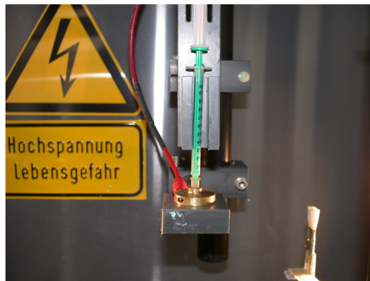
Figure 5.5: Close-up of self-made apparatus for electrospinning, located at Marburg
