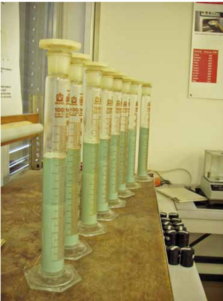
Figure 2 2 Determination of Zeleny sedimentation value: Flour is suspended in bromophenyl-solution (right four cylinders) and afterwards in lactic acid (left four cylinders) during 5 min in each step. Source: Isabell Hildermann
