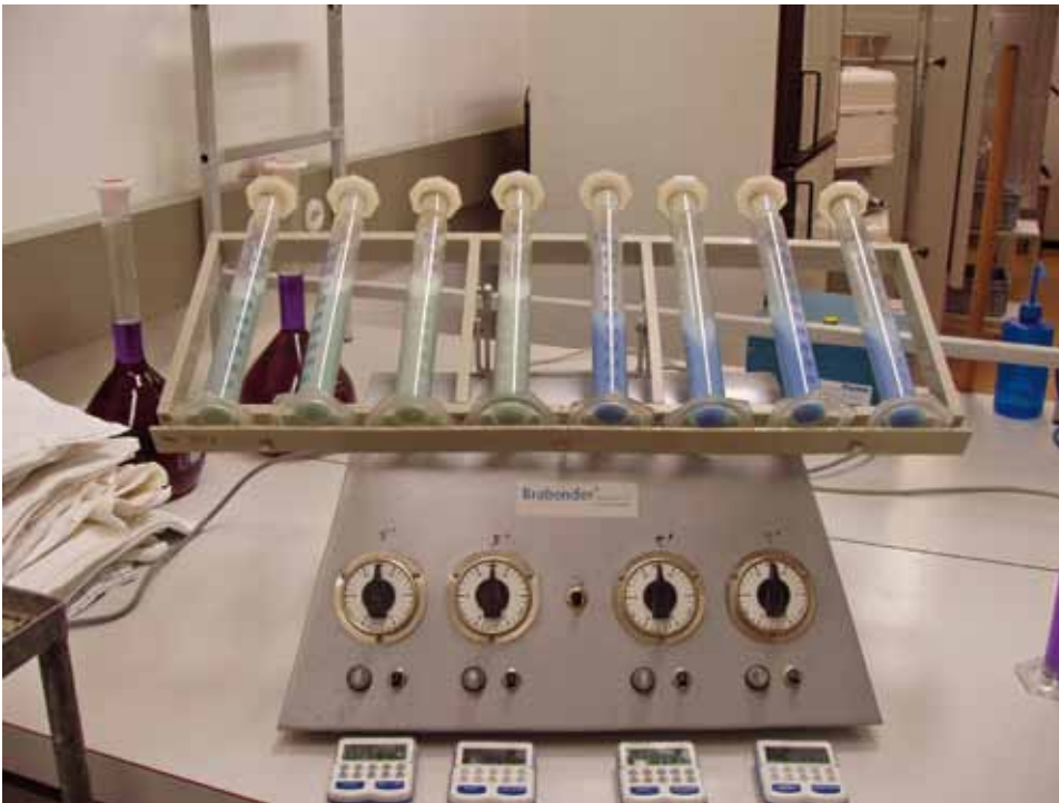
Figure 2 2 Determination of Zeleny sedimentation value: Flour is suspended in bromophenyl-solution (right four cylinders) and afterwards in lactic acid (left four cylinders) during 5 min in each step. Source: Isabell Hildermann
