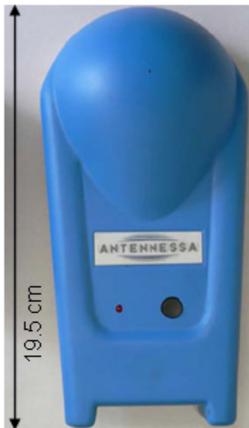
Figure 2-2: The exposimeter EME Spy 120
