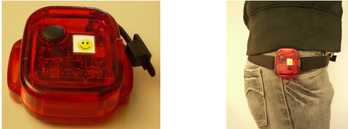
Figure 2.2 Actigraph Accelerometer (left), worn on the right hip (right)
