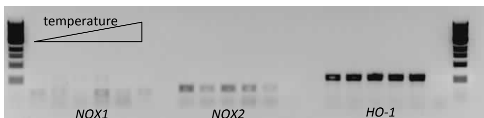
Figure 12. NOX1 , NOX2 and HO-1 PCR products at different annealing temperatures, loaded on a 1% agarose gel with a 1 kbp ladder.
