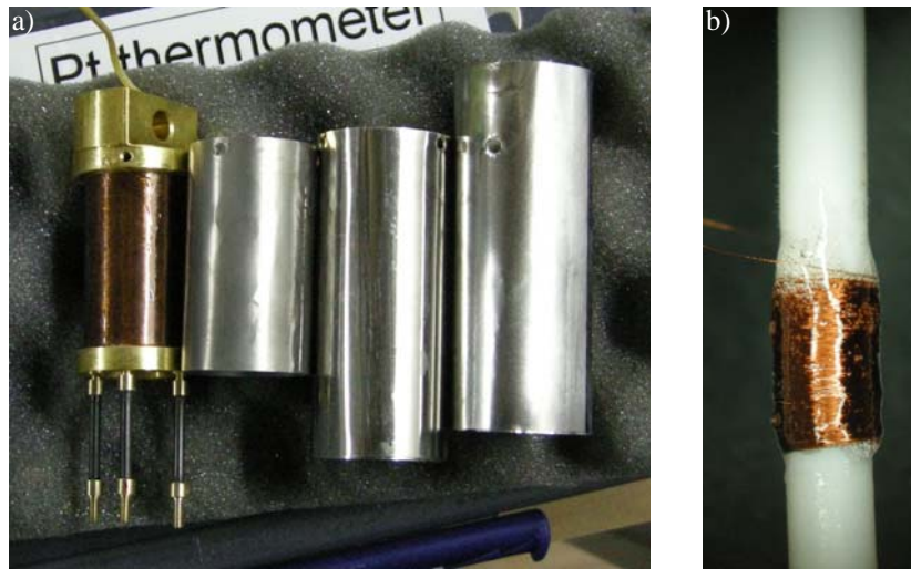
Figure 7.4.: Improvements that we tried. a) Extended niobium shields. b) A home-built coil wound on a Teflon former.
