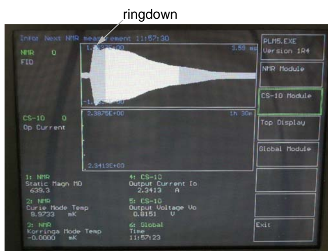
Figure 7.6.: Photograph of the PLM-5 display showing a free-induction decay of the platinum.
