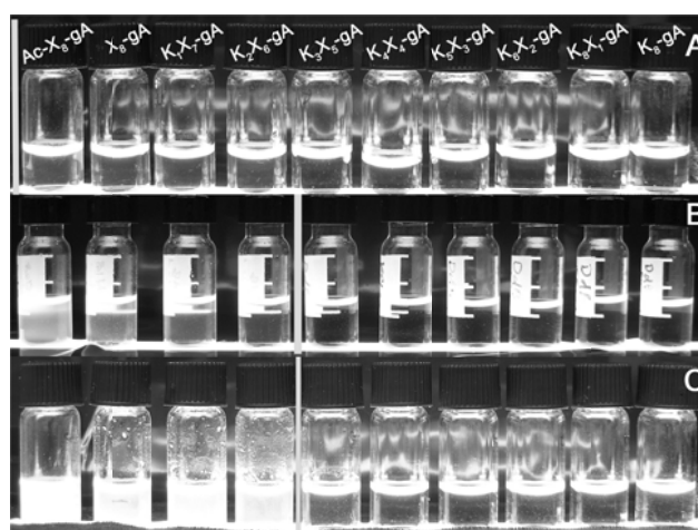
Fig. 5.3 Solubility of the amphiphiles in A) DMF B) ACN/water (1:1) C) ethanol.
