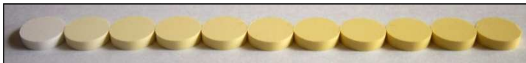
Figure 65: 1 tablet of each of the 11 batches of folic acid tablets, from 0% (far left) to 5% (far right) API
