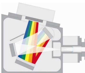
Figure 5: Diffraction grating NIRS. The incident light is first collimated by a concave mirror and guided on to the diffraction grating, where it is spatially split into its different spectral components. A second concave mirror focuses the various spectral components of the light onto different columns of the CCD detector, thus capturing the light's spectrum in a single acquisition.
