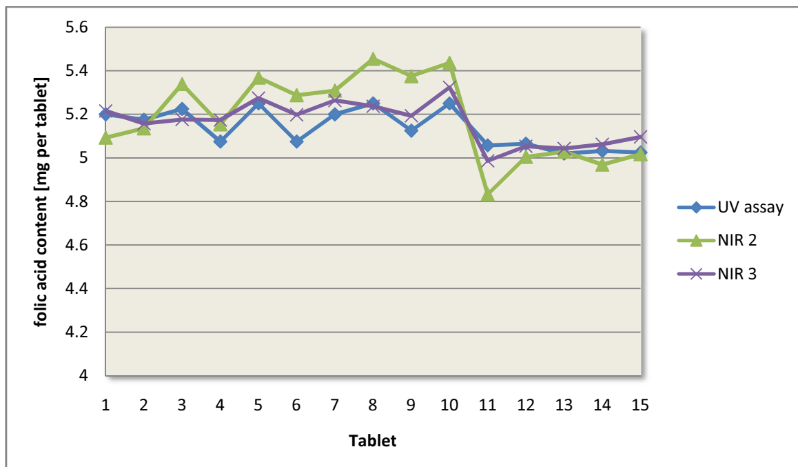
Figure 78: Prediction of variable compaction speed tablets by two NIR models, compared to the UV assay content
