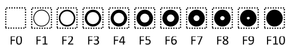
Figure 16: 10-mm printed rings used to produce a block effect. The number indicates the internal diameter in mm. The block from each filter to that from F0 was used to calculate block percentage.
