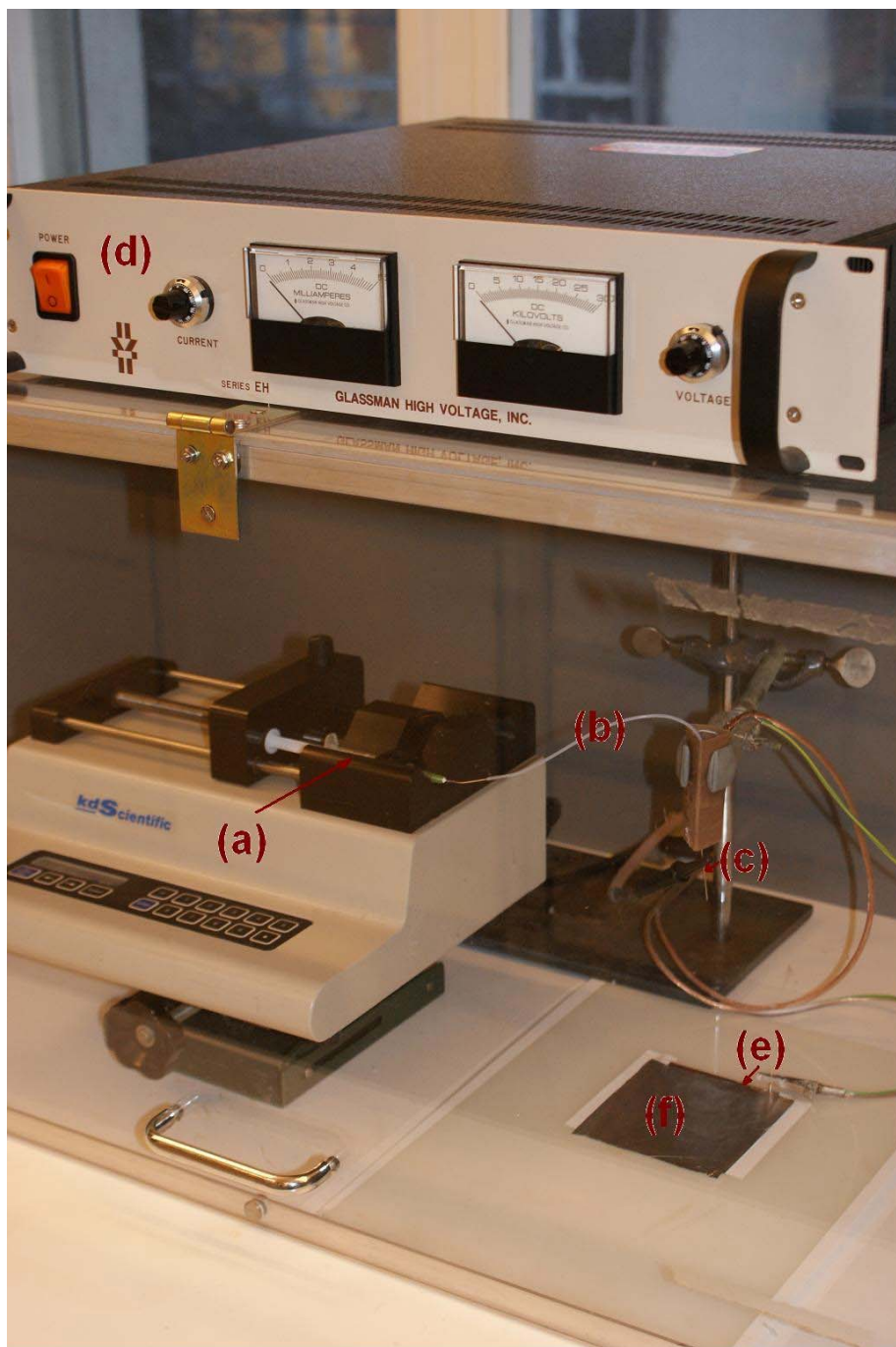
Figure 3.1: Homemade electrospinning setup with (a) syringe pump with syringe, (b) Teflon tube, (c) needle/capillary connected to high voltage, (d) high voltage supply, (e) grounded collector, and (f) aluminum foil.
