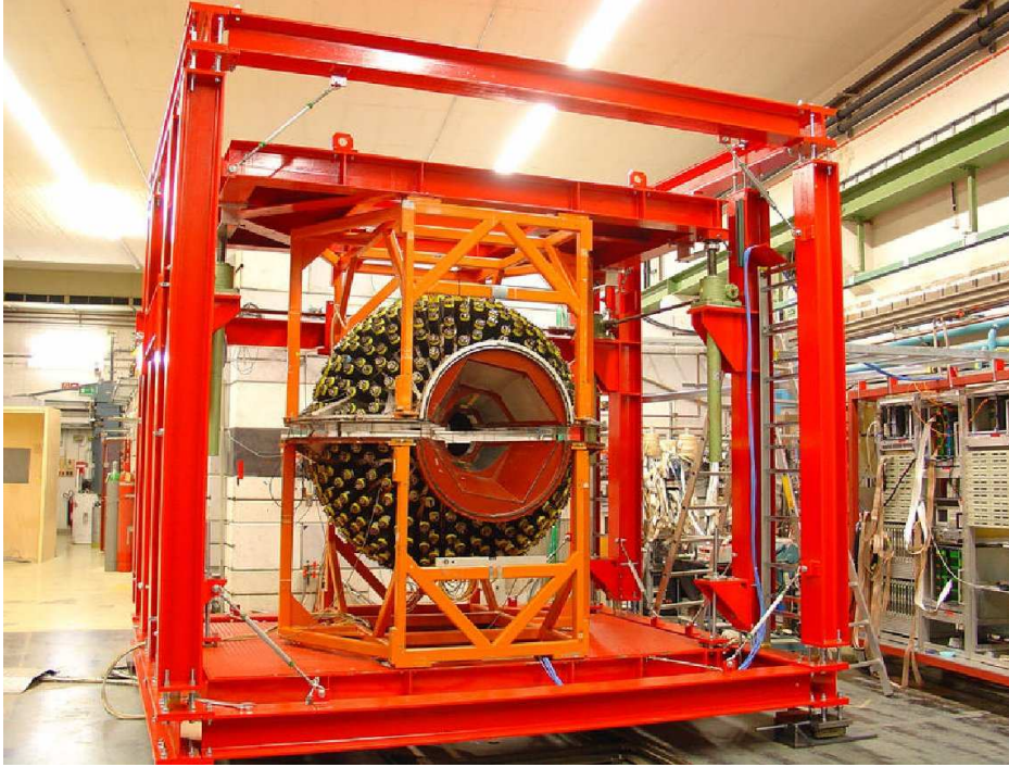
Figure 3.6: CB and its photomultipliers before cabelling
