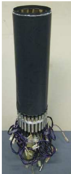
Figure 3.10: The PID detector before it is placed inside the CB.
