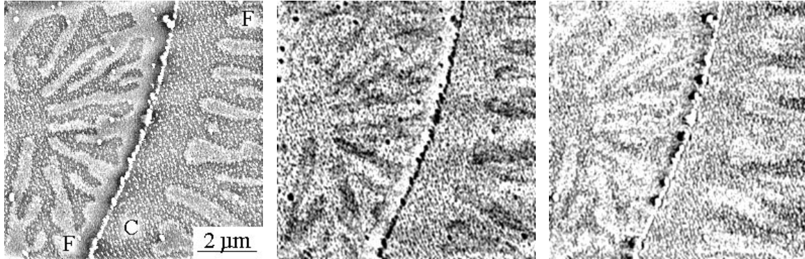
Figure 2.25: LEFT: \text{BaCuO}_2 flux structure with a fractal boundary line (SFM topview image). Note that the step in the middle of the image is decorated with small particles.
