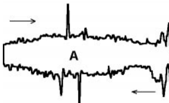
Figure 2.17: Friction loop of the topography scanline marked in white above. No contrast is seen in the friction signal irrespective of step edge contrast (sharp peaks). 'A' denotes the position of the platelet.
