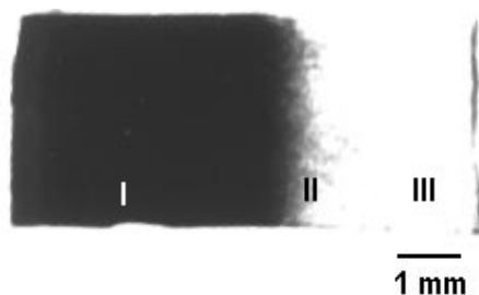
Figure 3.4: Photograph of a thickness-gradient film as prepared by the half-shadow technique described above (YBCO film on \text{LaAlO}_3 ). (I) – (III) see above.
