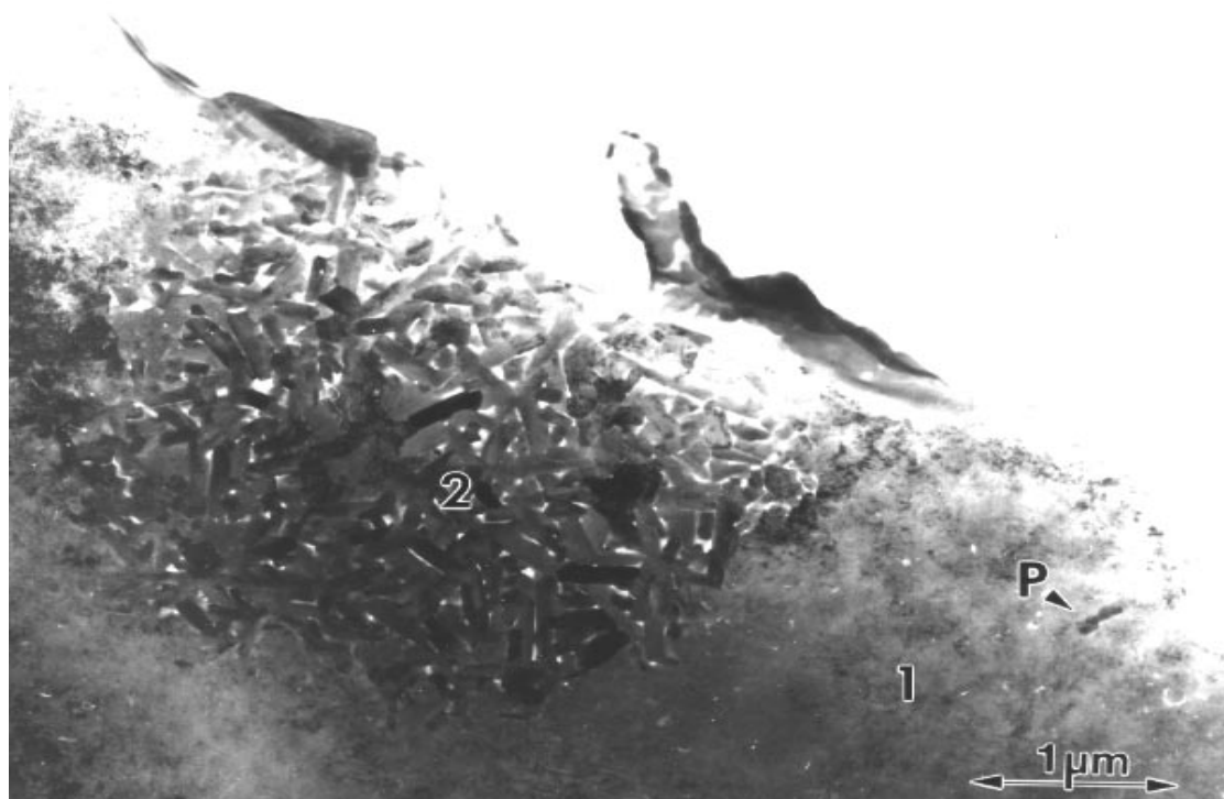
Figure 3.37: TEM image of a YBCO thin film on MgO(100). Most of the film is YBCO(001) '1', but a small area (labelled '2') close to the etched hole (upper right corner of the image) exhibits (100)-oriented platelets. An individual platelet is marked by 'P'.
