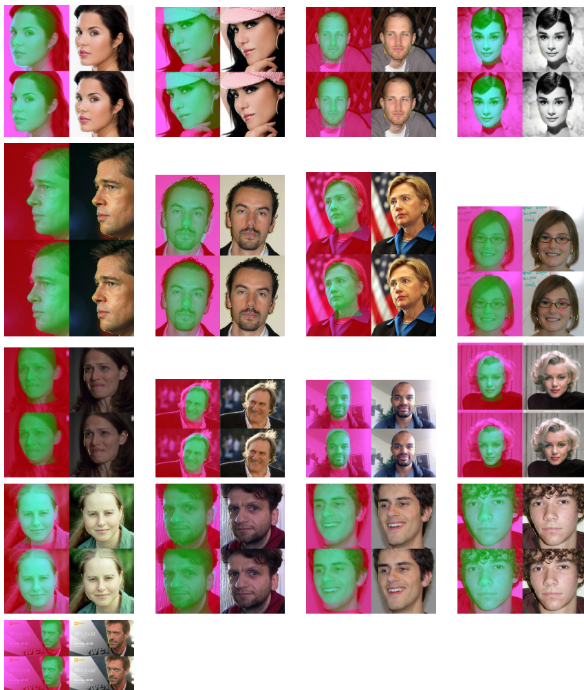
Figure 6.3: Failed silhouette extractions. The problematic cases either are lighted from behind resulting in a glow around the edges, have a background color which equals the face color, or have hair completely occluding the ears. The figure shows for each failed example the model fit after landmark fitting, the first extracted silhouette, the model fit after the sixth fit to the silhouettes, and the final extracted silhouettes.
