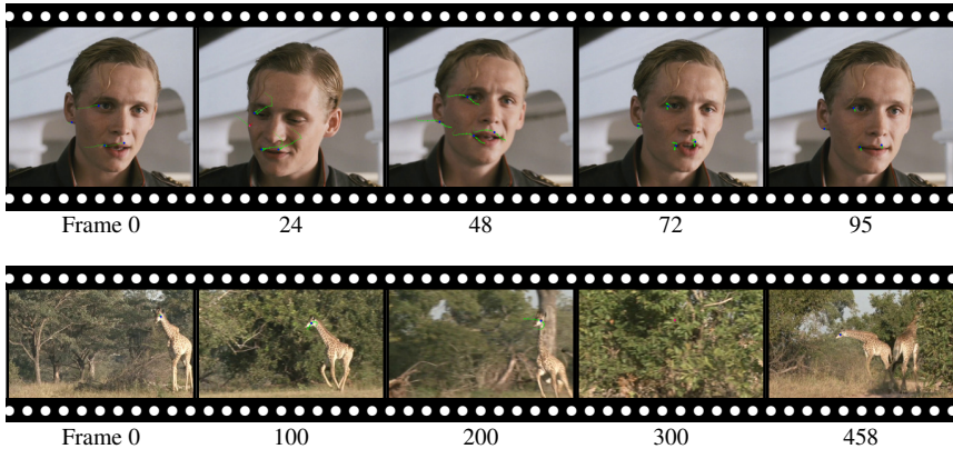
Figure 5.2: Tracking results on a talking head sequence and on a video of a giraffe. Between one and three user clicks were needed to achieve accurate tracking for the head sequence. Note the correct handling of the occluded ear, which was achieved with a single click. The eye of the running giraffe needed eight clicks, of which three marked occlusions. Please refer to the accompanying video for more details.
