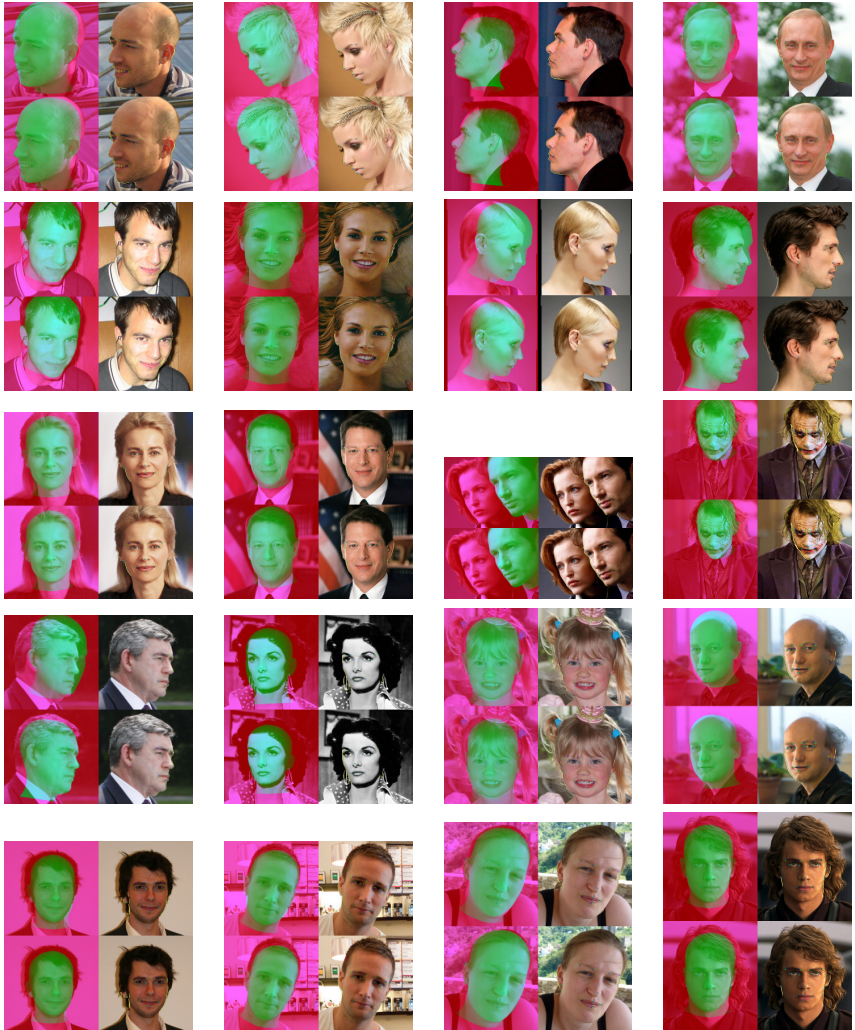
Figure 6.4: Some successful silhouette extractions. In most cases silhouette extraction returns few false positives, and allows the fitting to converge on the correct silhouette. We picked a few examples which were difficult because either the initialization was relatively far from the solution, the background color and foreground color were similar or the background has strong edges. All failures to converge are shown in figure 6.3
