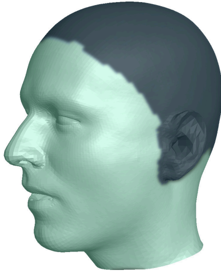
Figure 3.14: When registering an expression scan we are using the corresponding neutral scan as the template, and increase the stiffness in the area marked blue in this figure.
