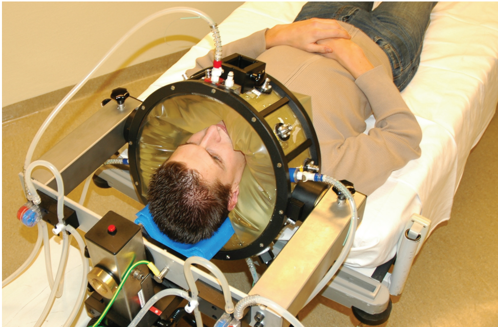
Figure 11.1: Head and neck hyperthermia applicator HYPERcollar developed at the Hyperthermia Group of Erasmus MC (Daniel den Hoed Cancer Center), Rotterdam, the Netherlands.
