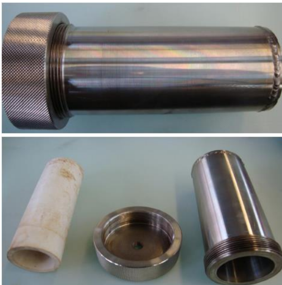
Figure 3.2: Autoclave used for hydrothermal synthesis
