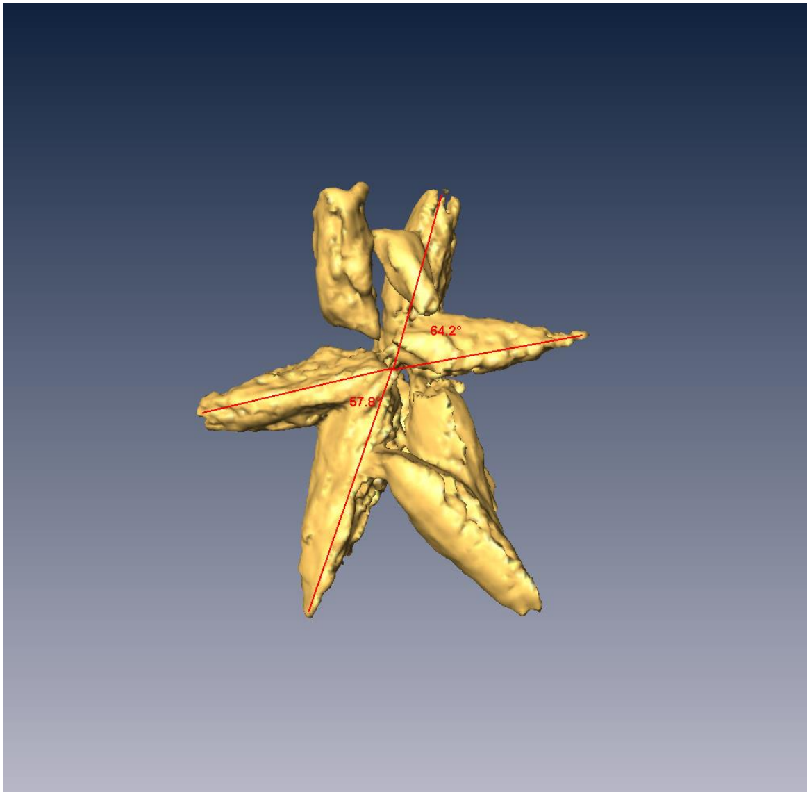
Figure C-6: STEM tomography of hematite nano flower showing the two dimensional geometry. [Courtesy: Dr. Rolf Erni, Mr. Daniel Schreier, Dr. Magdalena Parlinska, Electron Microscopy Center, EMPA]
