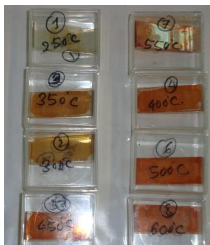
Figure 6.2: Hematite thin films obtained by the spin coating of polymeric precursor solution and heat treated at different temperature.
