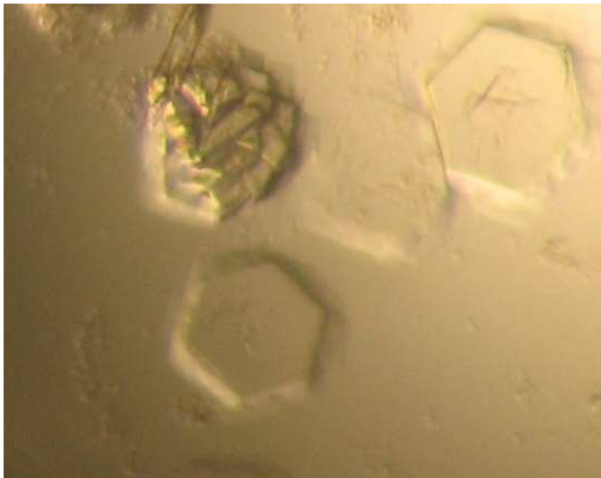
Figure II.1: OmpF crystal with hexagonal morphology belonging to space-group P321 (top) and C222 1 (bottom)
