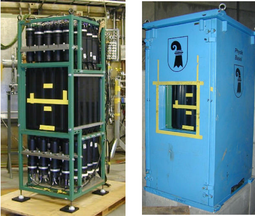
Figure 7: The left picture shows the neutron detector from the front. On the right side the neutron detector in the lead house is shown from the front
