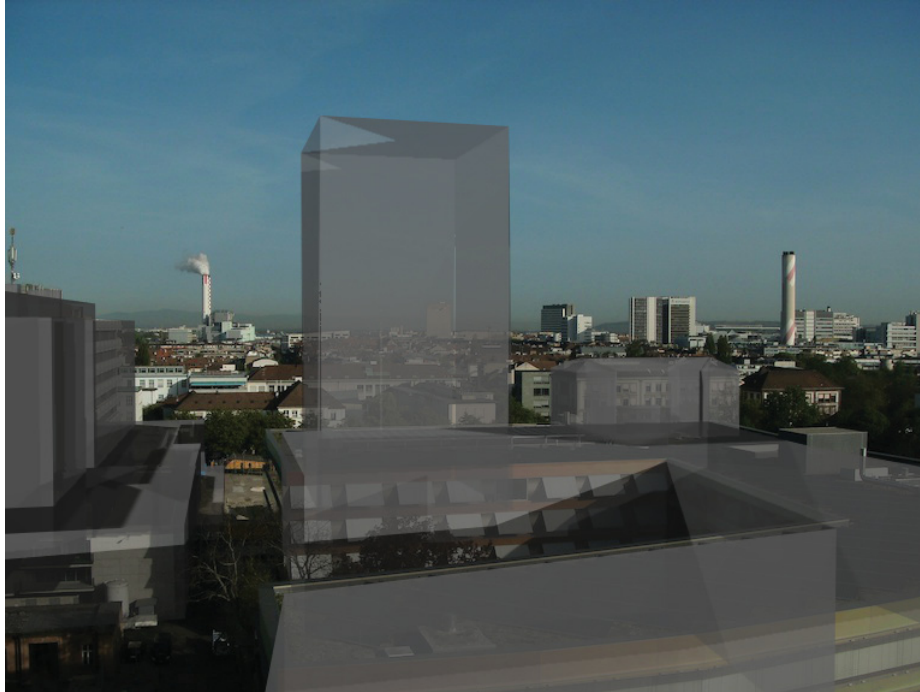
Figure 81: Hybrid image showing environment of the new building. The new building, as well as surrounding buildings that may from some perspectives occlude the future building, are rendered as partially transparent gray volumes (Image: F. Müller)
