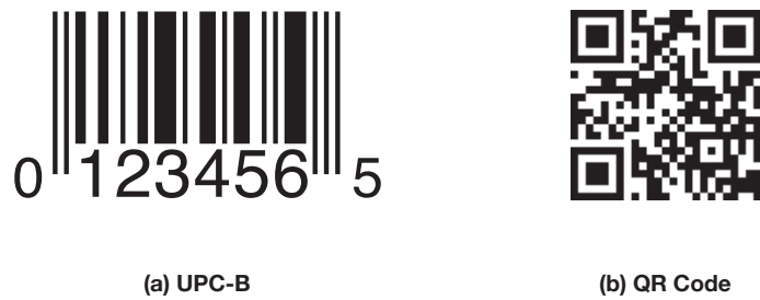
Figure 10: Comparison of one- and two-dimensional barcodes. The one-dimensional Universal Product Code (UPC-B) in subfigure (a) encodes information in the horizontal dimension, the two-dimensional QR-code in subfigure (b) encodes information both in the horizontal and vertical dimension (Image: F. Müller)
