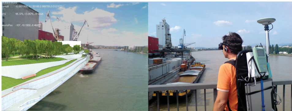
Figure 71: Live view from the Lifeclipper2 system (left) and user wearing the system on his back (right)
