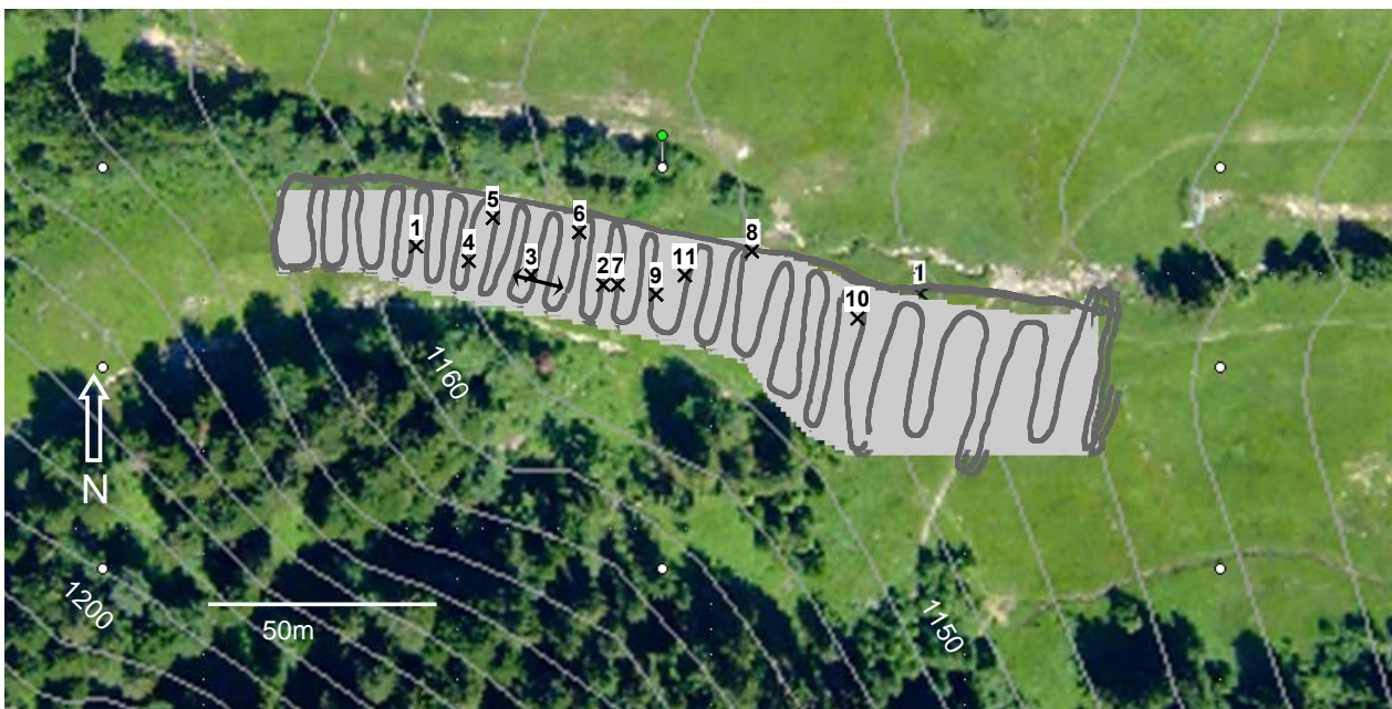
Figure 2 Satellite photo with contour lines and test field (grey) with raw data distribution from EMI survey, in this case March (dark grey line), the location of the soil samples (black crosses) as well as the location of the FDR transect (double arrow)
