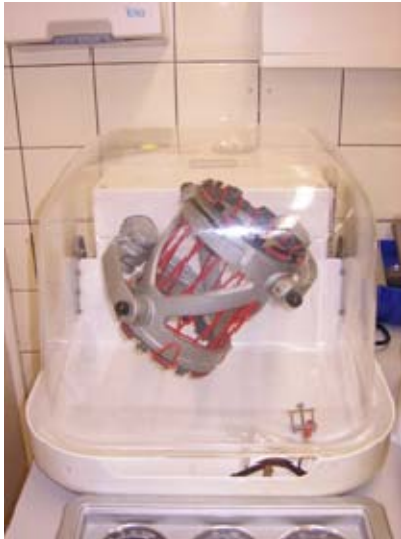
Figure 36. Turbula mixer (Type T2A, Willy A. Bachofen, Basel, Switzerland).
