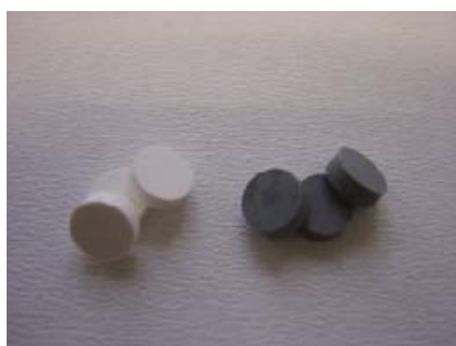
Figure 47. Tablet before and after using a mercury porosimeter.
