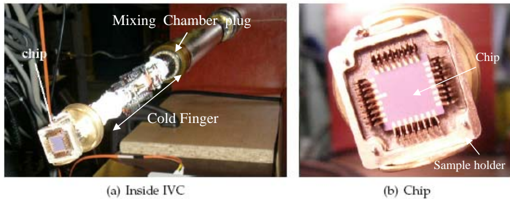
Figure 3.6: Cold finger, socket and sample holder
