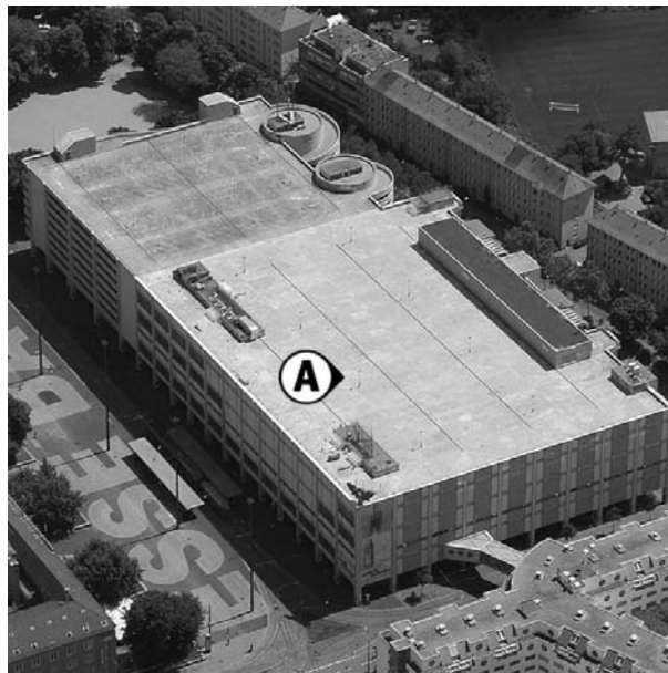
Figure 3.11: Aerial photo of site Basel-Messe (U3) located on a large concrete roof. The marker 'A' indicates the location of the sonic and radiation instrumentation. Photo by courtesy of R. Vogt, University of Basel. View from NW.
