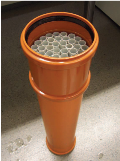
Figure 3.1: Structure phantom consisting of 43 tubes of 13 mm in diameter each. The tube phantom, 130 mm in diameter and 650 mm in length, was built to model a patient's arm.
