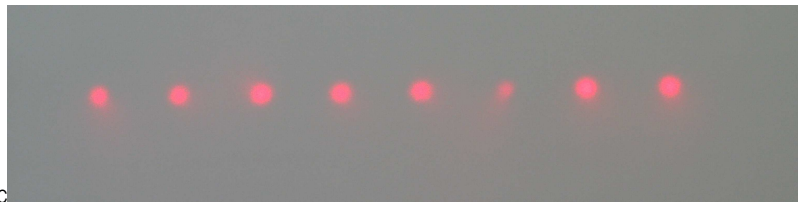
Date Image Laser Lens I Lens I Orientation Lens II Lens II Orientation 27.04.2010 IMG_0410.JPG 8x Bestform f25 MellesGriot Laser -> (| Plano-conv. f50 Laser -> |)
