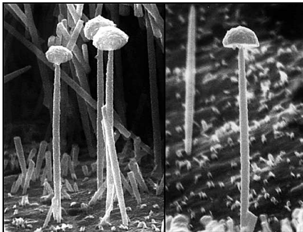
Figure A.1: SEM images of electrochemically grown Ni wires in template after its dissolution (wire length \sim 6 \mu\text{m} , apparent diameter 100-280 nm).
