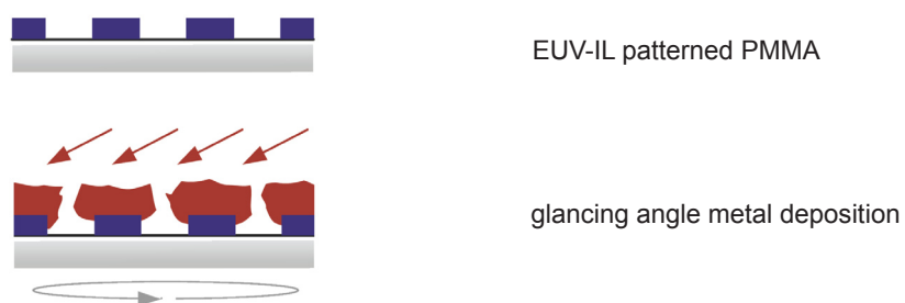
Figure 3. Scheme of evaporation of additional Cr/Ag mask upon EUV structures using glancing angle deposition (GLAD) technique (10).
