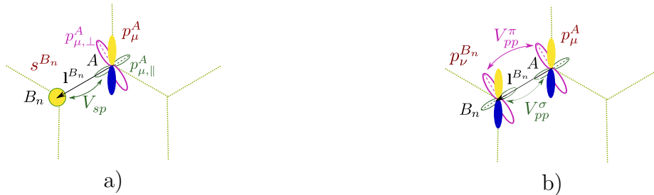
Figure 3.4: The hopping element between a) p_\mu^A and s^{B_n} b) p_\mu^A and p_\nu^{B_n} can be calculated by the decomposition of the p_\mu^A(p_\nu^{B_n}) orbital into two parts: perpendicular to the bond p_{\mu,\perp}^A(p_{\nu,\perp}^{B_n}) and parallel to the bond p_{\mu,\parallel}^A(p_{\nu,\parallel}^{B_n}) .
