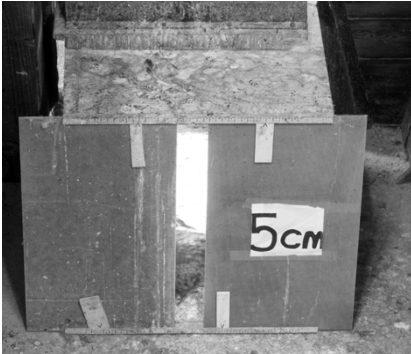
Figure 2. Experimental design with a tunnel and adjustable wooden boards to test the minimal restriction a feral pigeon is able to pass through. In this experimental design the width can be varied to the extent that even a highly motivated pigeon is not able to squeeze through the opening.
