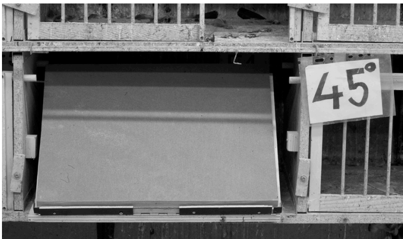
Figure 4. With a holder fixing the test material, here a sandstone slab, the maximal inclined slope a feral pigeon can sit on was tested.
