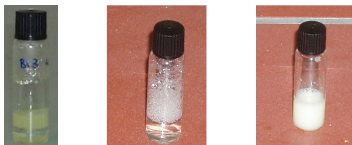
Figure 4-1 Appearance of the reaction mixture of the conjugate addition reaction of butanal to nitrostyrene in water in the presence of 1a (left), of an aqueous solution of peptide 1b before (middle) and after (right) the addition of butanal and nitrostyrene.
