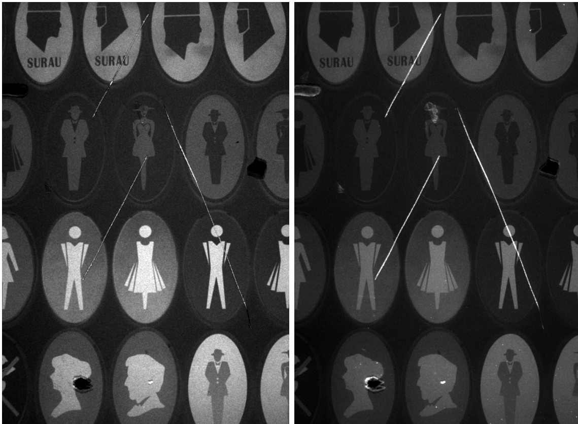
Figure 8.1.2: Images acquired with 50^\circ angle in simple dark-field setup (left) and in polarized dark-field setup (right)
