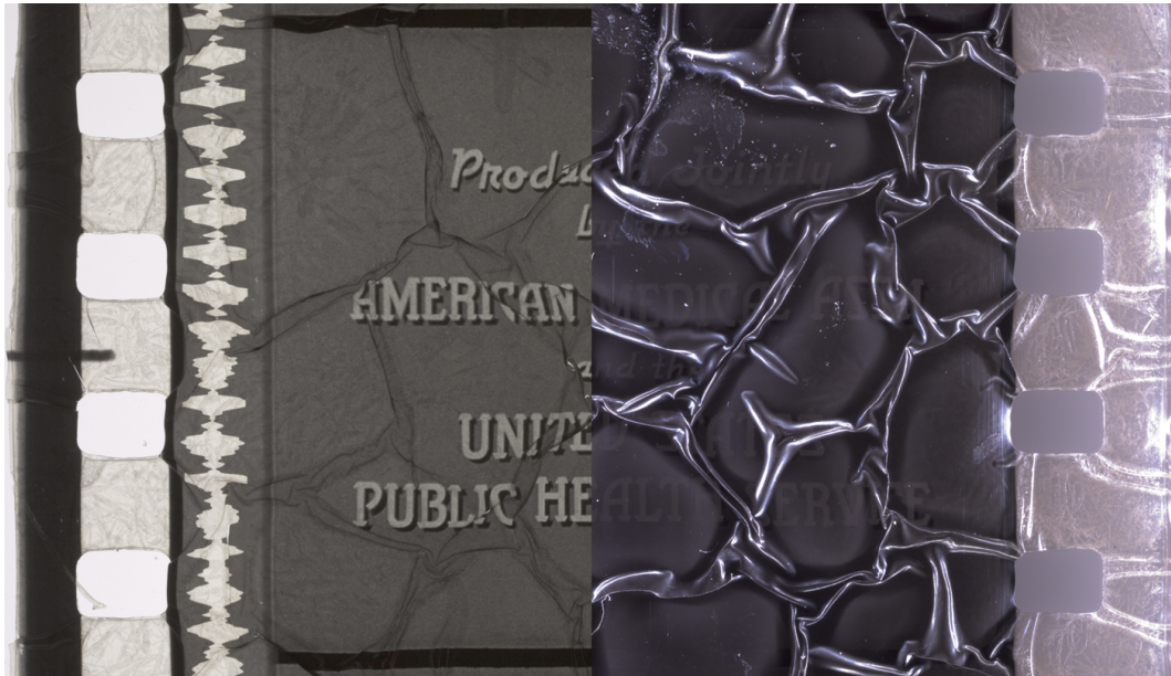
Figure 5.1.10: A film affected by vinegar syndrome illuminated in bright-field (left) and with raking light (right) (sample source: Image Permanence Institute - digitized by the author)
