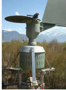
Figure 3.4: Burkard pollen sampler mounted on the towertop north of the pollen source.
