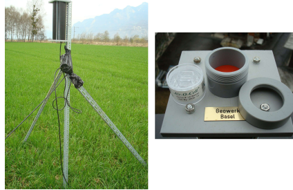
Figure 3.5: Mounting of the AOC pump (left) and AOC cassette and its fixture in the pump (right).
