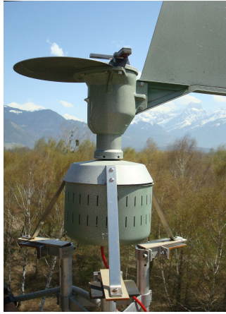
Figure 3.6: Burkard pollen sampler mounted on the towertop north of the pollen source.
