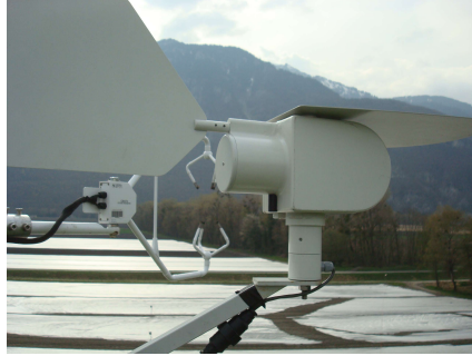
Figure 3.7: Burkard Sc. mounted on the towertop south of the pollen source with the CSAT3 ultrasonic anemometer in the background.
