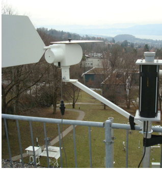
Figure 3.10: Set-up of inter-comparative measurements in Zurich. On the left the Burkard Sc. and on the right the AOC system is displayed.
