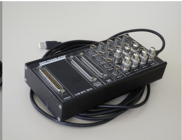
Analog Digital Converter Unit Data Translation® DT9804
