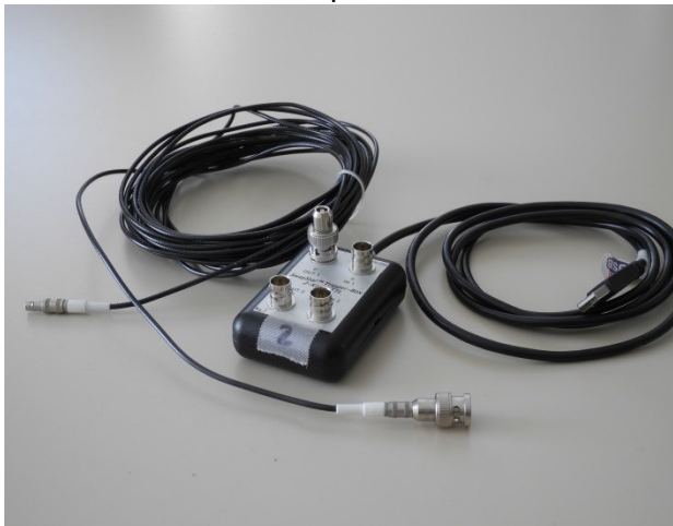
Trigger Unit based on FTDI RS232 to USB Adapter
