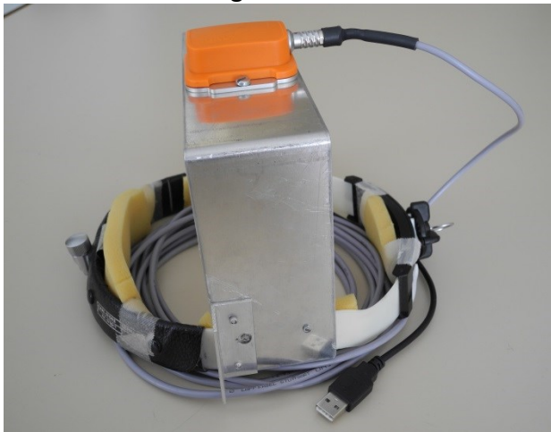
MTI Xsens Sensor Unit on Headband Mounting
