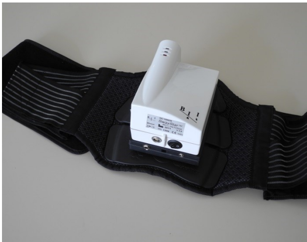
SwayStar™ unit on converted motor-cycle kidney-belt
