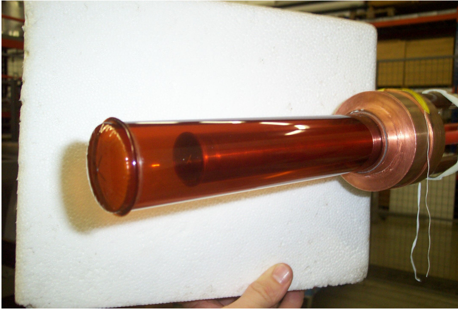
Fig. 2.4: Photo of the liquid hydrogen/deuterium target cell. Taken from [50].
