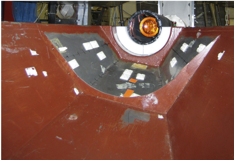
Fig. 4.24: Photo of the Crystal Ball exit tunnel region including target cell and PID detector: The complex geometry of the beam exit tunnel is at the moment not exactly modeled in the simulation.
