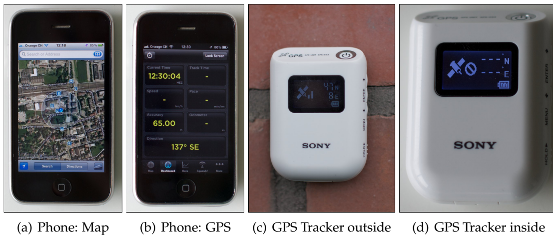
Figure 10.45: Devices for tracking the position while taking pictures: (a) shows a smartphone with built-in GPS. The application shows the position on the map; pictures taken with the smartphone camera are automatically tagged with the position. Running a different application as displayed in (b), the same smartphone can log the position to create a track that can later be used to tag images taken with a different device via timestamps. The same functionality can be provided with a dedicated device like the one shown in (c). However, this only is possible as long as the GPS signal is received. In (d), this was not possible while being inside a building.
