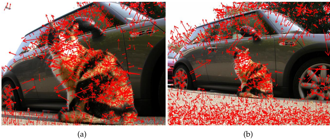
Figure 10.77: Keypoints in images: The 1481 SIFT keypoints extracted from the query image (a) and a very similar image of same size with 2536 keypoints (b) to which we will later on compare it.
