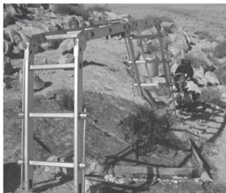
Fig. 5. Portable nozzle simulator during rainfall simulation test.
