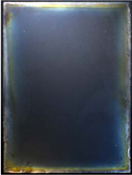
Figure 6. Silver gelatin glass negative. Cueni study collection (~1910). Silver mirroring with bronze and greenish colour.
