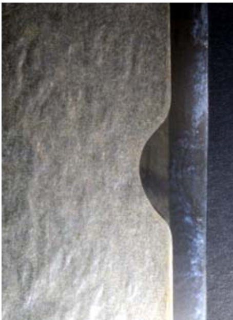
Figure 19. Silver gelatin glass negative. Cueni study collection (~1910). Lines of mirroring similar to the rounded opening of an envelope. For purpose of showing this effect, the plate is shifted to the right
