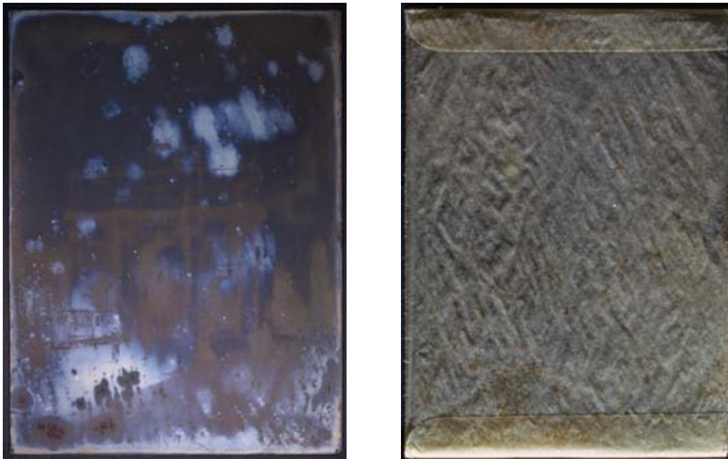
Figure 17. Silver gelatin glass negative. Cueni study collection (~1910). Spots and stains of silver mirroring connected with brown marks on the glassine envelope (b) in which the plate was stored.
