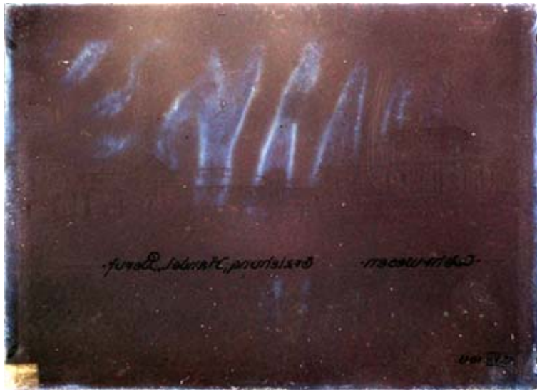
Figure 1. Silver gelatin glass plate, Schweizerische Landesausstellung collection (~1914) Swiss State Archive. Silver mirroring stains similar to the creases of the glassine enclosure.
