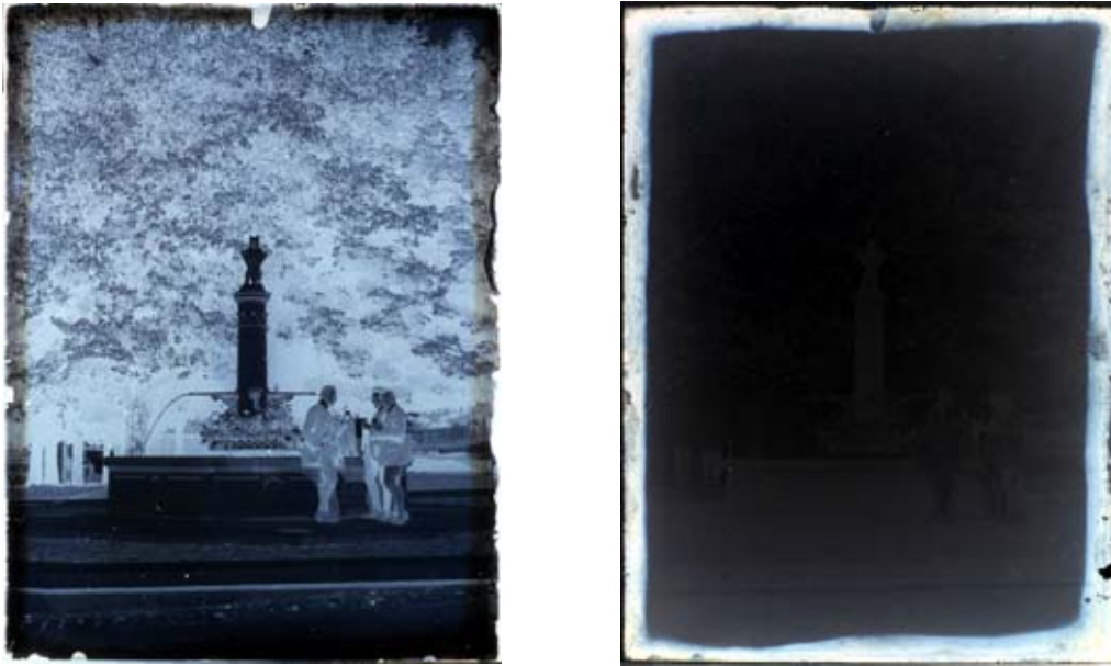
Figure 9. Silver gelatin glass negative. Cueni study collection (~1910). The comparison between the photograph in transmission (a) and in reflection (b) shows that the silver mirroring intensity is the same in the low-density (tree leaves) and high-density (ground) areas.
