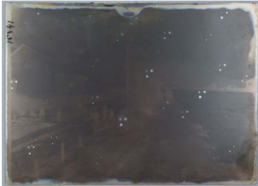
Figure 18. Silver gelatin glass negative (courtesy of S. Dobrusskin). Three-spot pattern of silver mirroring at the centre of the plate. Along the upper side the shape of the mirroring stain matches the rounded opening of a sleeve.
