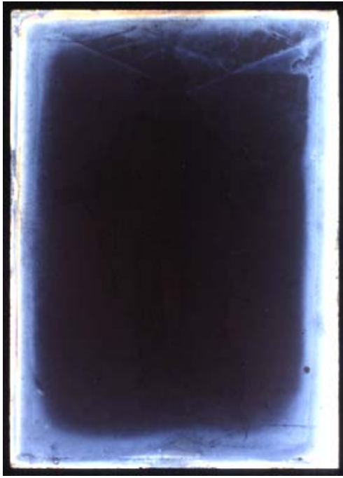
Figure 13. Silver gelatin glass negative. Cueni study collection (~1910). Lines of silver mirroring similar to the folds of an envelope.
