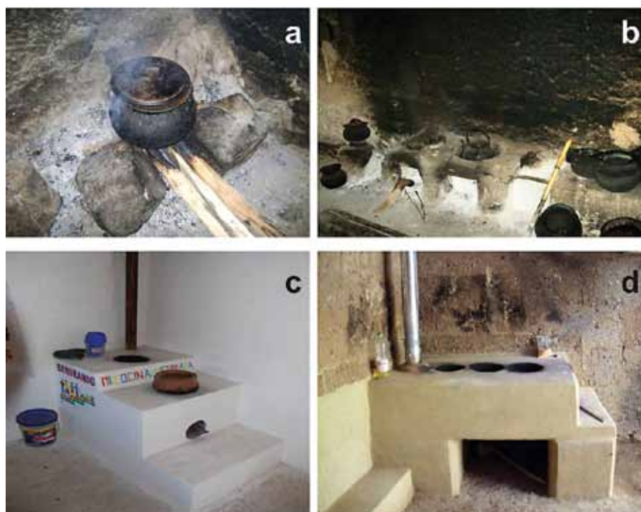
Figure 1. Type of stoves found in the Province of San Marcos and the OPTIMA-II improved chimney stove model. a: Open fire “Tulpia”; b: “Traditional” stove; c: government design “SEMBRANDO” stove; d: OPTIMA-II stove.
