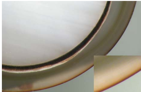
Figure 2: Cross-section of a 'chocolate' beaded cultured pearl. The light-coloured bead (i.e., nucleus) and the darker overgrowth are clearly visible. It is evident in the enlarged image at the bottom right that the brown colour has been artificially added. This demonstrates the porosity of a cultured pearl and its potential for absorbing chemically doped or colour-doped solutions. The colour has penetrated approximately 0.5 mm. Photo by H. A. Hänni.
