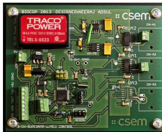
Figure 3.10: - Implemented board of SUPERAMP. Third channel is not soldered.
