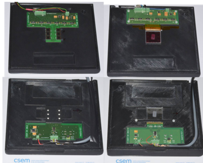
Figure 4.21: - Photos of the 4 distinct PCBs: driving electronics for inorganic LEDs, driving electronics for OLEDs/LE-FETs, detection electronics.
